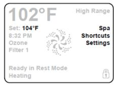
Rest Mode will only allow heating during programmed filter cycles. Since polling does not occur, the temperature display may not show a current temperature until the filtration pump has been running for a minute or two. Ready in Rest Mode may appear when Jets 1 is activated.
